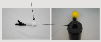
Then connect your ½" tubing lines (VL0140) to each "Y" connector (both ends as pictured), and run the lines along the boom frames toward the tank/compressor assembly. Cut your tubing accordingly for each line. Make sure there is excess tubing where your spray boom folds up to prevent the lines from getting tangled.
