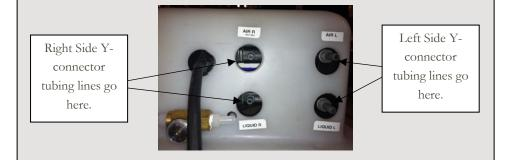
Finally, secure the tubing lines along the boom and sprayer frame with the nylon ties provided (NY108H). Be careful to not kink or pinch the lines with the ties provided. You should be ready to go! Make sure that your push to connect power chord is connected, and then follow our operating instructions to start making foam.
