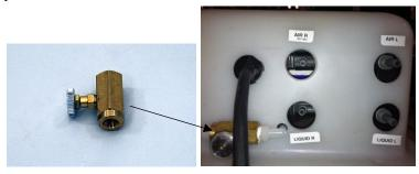
Note: If the needle valve is opened too far, the foam chambers will flood and produce wet, sloppy foam. You should be able to produce a drop every second if you adjust the nozzle to optimum speed. In most spraying applications this is more than enough marks per foot. You can conserve your foam by turning down the liquid flow when a desired foam consistency is achieved.
