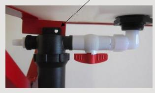
Attach your pump assembly and mounting bracket (WWTC01) to your 3-point hitch model in the position pictured with the U-bolts provided (NBUB07 QTY: 2).
