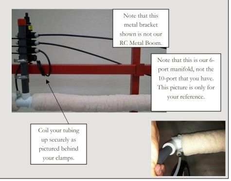
Step #8 Using the weed wiper with your sprayer and installing the electrical wire harness
