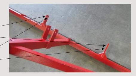
Secure your top lynch pin insert down with the <sup>3</sup>/<sub>4</sub>" x 4 <sup>3</sup>/<sub>4</sub>" RC link pin (WR4012 QTY: 1) and RC lynch pins (WR4010 QTY: 1). Follow the picture below.
