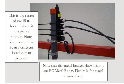
We provide the pump needed to power our weed wiper. We also provide the vinyl tubing needed to run from your manifold to your pump (VL0038 QTY: 6 ft.). The length required may vary based on where your pump is located in comparison to the center of your boom where your manifold has just been mounted. Now, connect your manifold to your spray pump.
