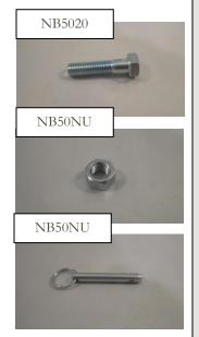
Attach your wings by inserting <sup>1</sup>/<sub>2</sub>" x 2" bolts (NB5020 QTY: 4) with <sup>1</sup>/<sub>2</sub>" Jam nuts (NB50NU QTY: 8) into the inserts as pictured (4 bolts per wing side). Insert the RC Wing Pin (WR4240 QTY: 2) to hold each wing into position at the desired angle. <u>Be sure to attach them so that your wing angle iron tabs</u> are facing the opposite direction of your toolbar angle iron tabs (see picture).
