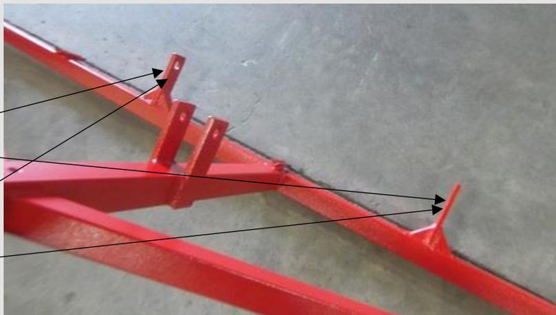
Secure your top lynch pin insert down with the ¾" x 4 ¾" RC link pin (WR4012 QTY: 1) and RC lynch pins (WR4010 QTY: 1). Follow the picture below.
