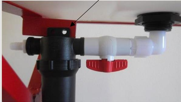
Attach your pump assembly and mounting bracket (WWTC01) to your 3-point hitch model in the position pictured with the U-bolts provided (NBUB07 QTY: 2).
