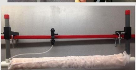
Any spray nozzles on your boom that are not in use, can either be switched to the off position, or capped with our cap and gasket shut off (SS-19843NYR QTY: 15). Attach a short piece of black tubing from your 1/4" tubing roll (WW1215 QTY: 90 ft.), from the TeeJet fitting to the inlet of the sponge section. The sponges and spray nozzles have an easy to use push to connect fitting that can only be released by pressing on the grey ring on the fitting, while pulling out the tubing.
