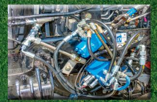
Raven Smartrax or Ag Leader Steer Command on a hydraulically steered 20,000# front axle.
